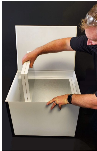
Insertion of EPS side panels.
